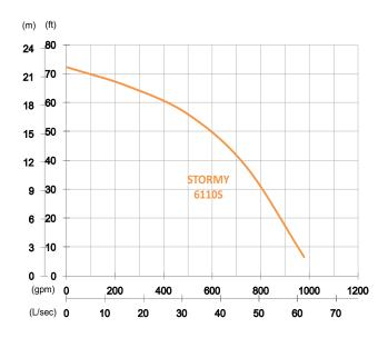
Shaft Speed: 1450 rpm Outlet: 150mm, 6in
